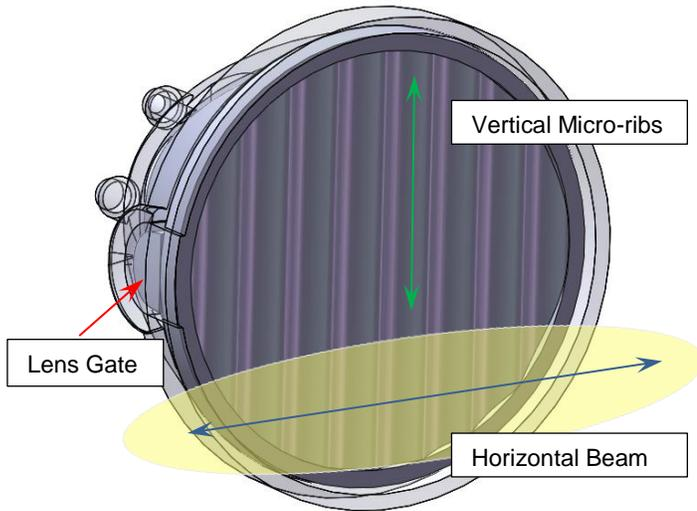
The elliptical lens produces a beam with its long axis perpendicular to the micro-ribbing on the lens face.
