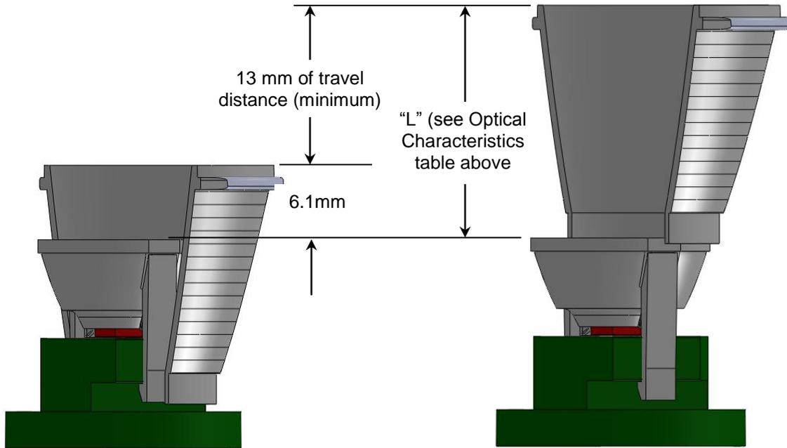
FXGR in Wide Flood position with larger reflector fully retracted
