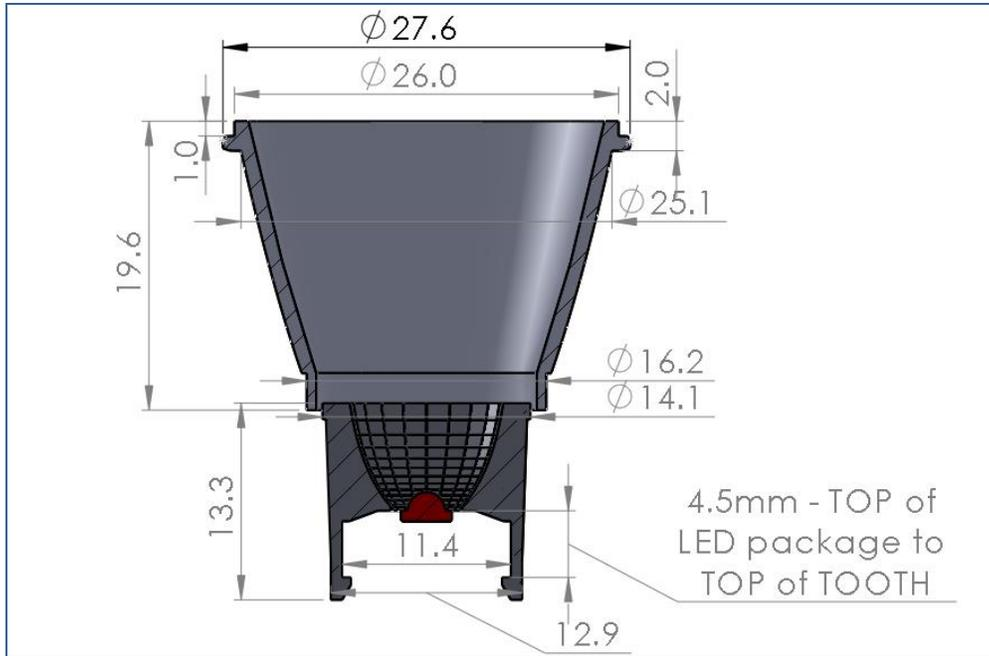
Figure 2. Mechanical dimensions of the FXGR Dual-Beam Focusable Reflector System
