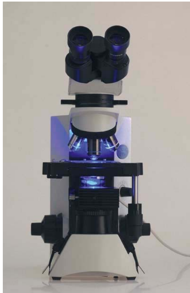
AFTER® fluorescence LED module on a CX 31 Olympus microscope
