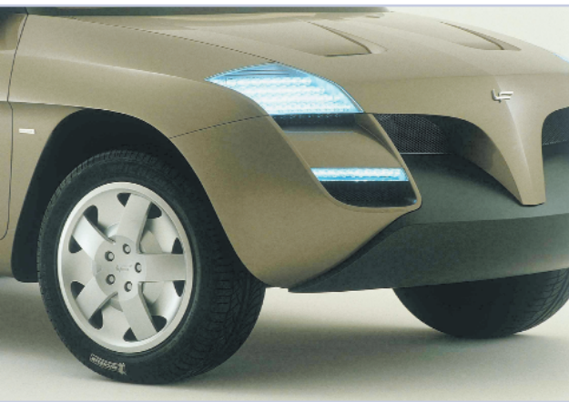
Car-designer Fioravanti's Yak concept vehicle demonstrates the potential of LED-style headlamps.
