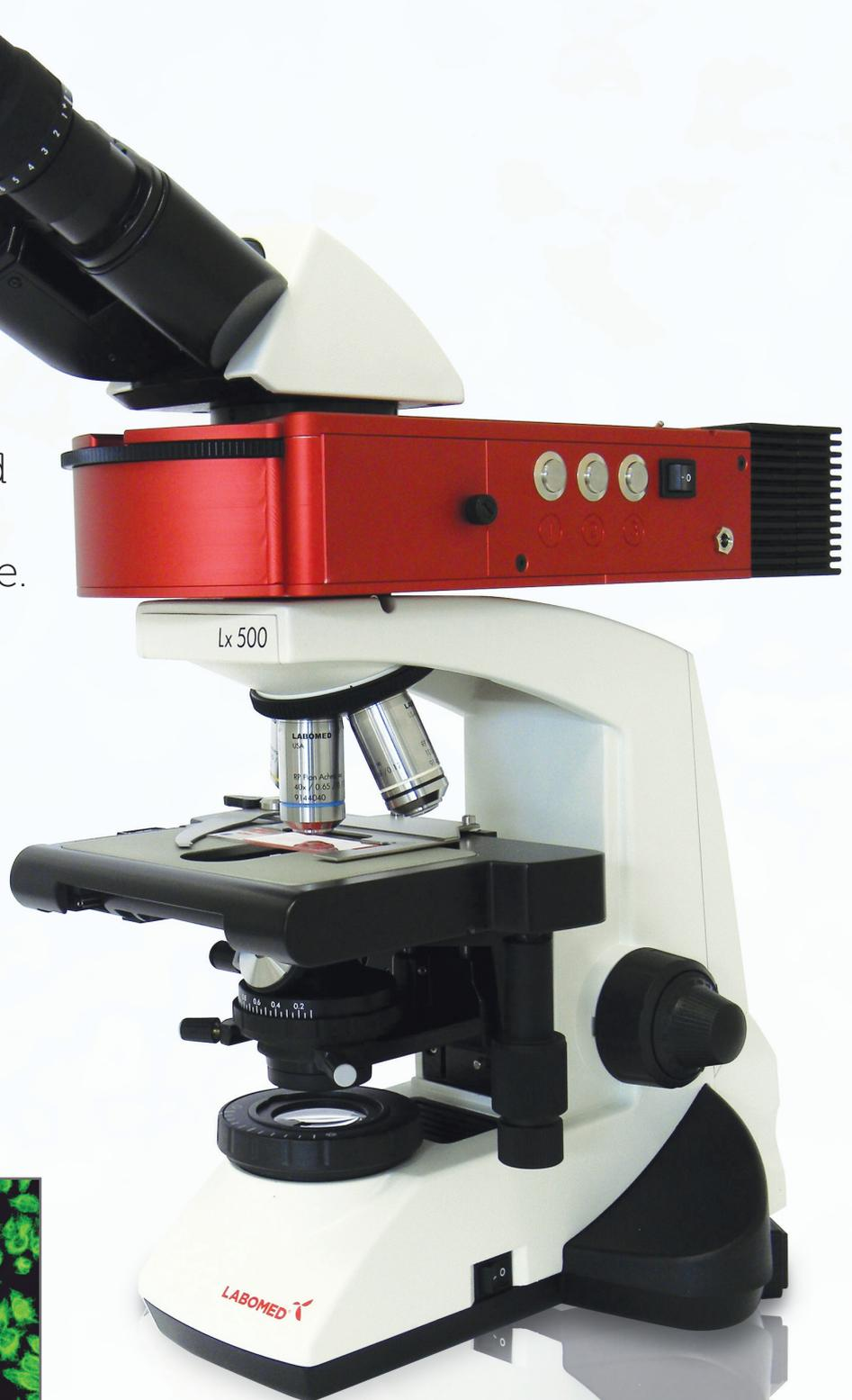
FLUOLED® 3CFW on Labomed Lx500 microscope.
