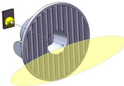
**Figure 3: Elliptical beam orientation**
