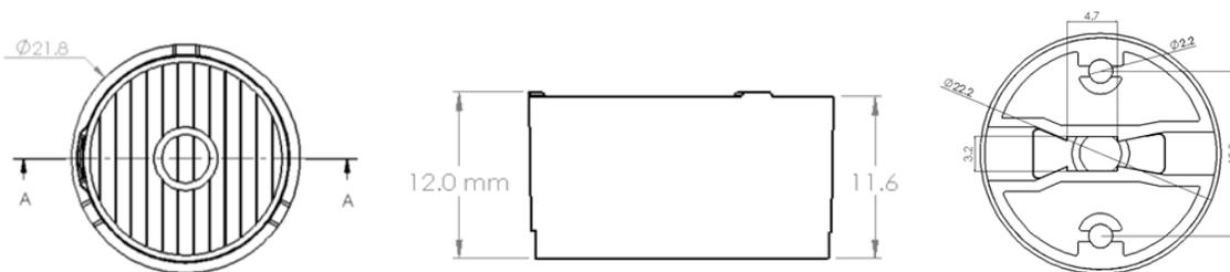
**Figure 5: Top, side and bottom assembly views with dimensions**
