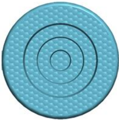
Narrow Beam Small, textured micro-lenses
