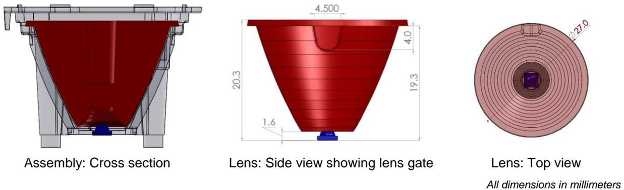
Figure 3. Showing relationships between the LED and a properly positioned lens
