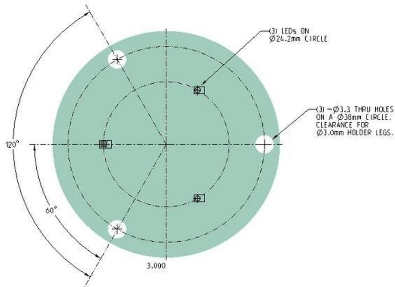
Figure 5: For proper fit of the FT3 tri-lens, the PCB should have thru holes and LEDs located as shown. The indicated LED position aligns the electrical contacts of the LED with the clearance channels in the lens holder.
