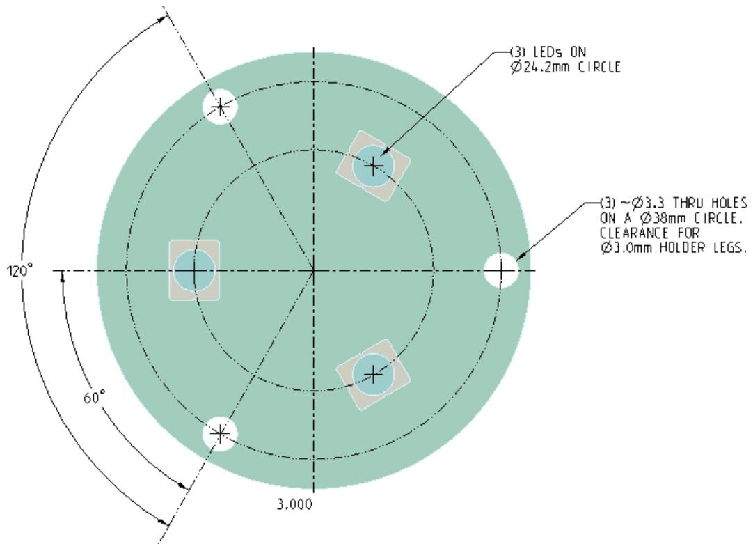
Figure 5: For best fit to the FS3 tri-lens, the PCB should have thru holes and LEDs located as shown above. The rotation/orientation of the LEDs should be as shown, for the LED wires to align with the clearance slots in the lens holder. This is also shown in Figure 2.
