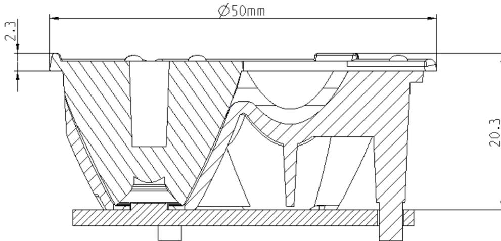
Figure 3: X-section view. The dimension “20.3 mm” represents the distance from the top of the lens holder to the bottom of the LEDs.
