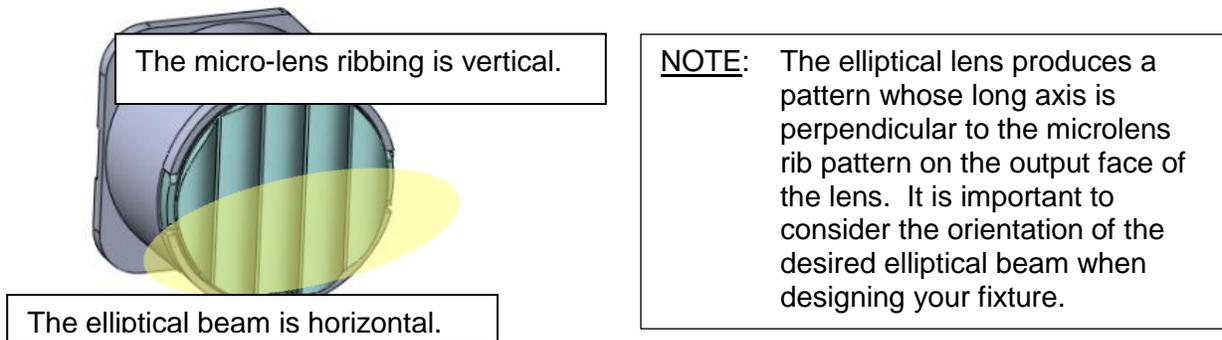
**Figure 4: Design considerations when using an Elliptical Lens**
