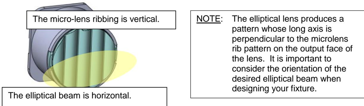
**Figure 4: Design considerations when using an Elliptical Lens**
