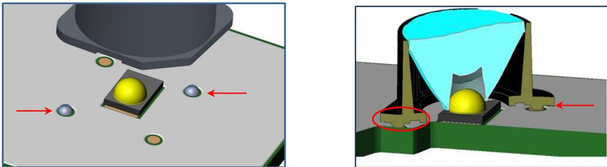
**Figure 6: FLT assemblies can be fastened to the PCB by placing a small drop of glue in one or more of the pin recesses on the board. When properly attached, the alignment pin rests in the board recess and the flat bottom of the assembly is in contact with the top of the PCB.**
