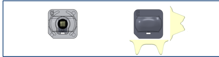
Figure 3: Note the relationship between the LED package, LED dome and the orientation of the FMT-E1 lens (left). The FMT-E1 lens delivers an asymmetric beam (right) with the wide, batwing profile being aligned with the long axis of the lens.
